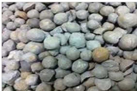
Gambar 3. Besi sponge hasil proses sintering
